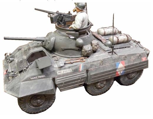
The crew of four comprised a commander (who doubled as the loader), gunner, driver, and radio operator (who could also act as a driver). The driver and radio operator were seated in the forward section of the hull, while the commander and gunner sat in the turret, with the commander seated on the right, and the gunner on the left.
