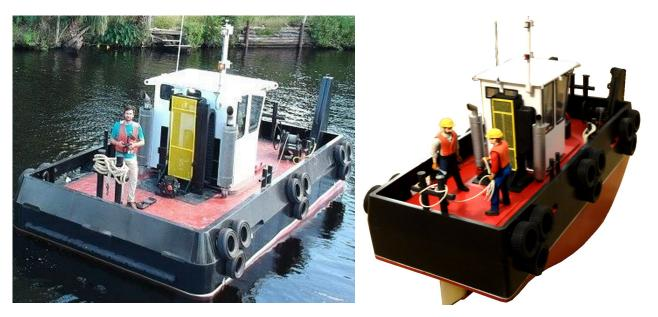
In the photos above, you can see where I had to "give" a little liberty to fit the real boat features in to the slightly narrower proportioned Springer configuration. The pilot house had to be a little narrower as well as the deck space on either side of the house.
