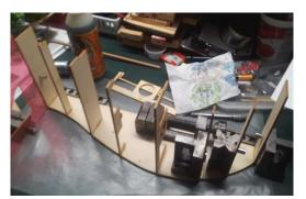
The "Tugsters" are an easy build model. (I have built many boats from scratch so I was not afraid of that option if I had decided to take that route.) All of the parts in the basic Tugster kit are plywood, 1/16, 1/8 inch and 1/4 inch thick. They come in the laser cut sheets and just need to be popped out using a small cut here and there. Everything went together very well. The instruction booklet was easy to follow and in very little time the hull was ready.
