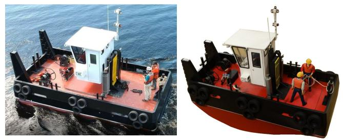
Above, the pilot house is in a middle position. The model also has a flexible "drag chain" (also 3D printed) located to the right of the yellow safety mesh that rolls as the pilot house moves. All 18 bumper tires were 3D printed and have great detail down to the treads.
