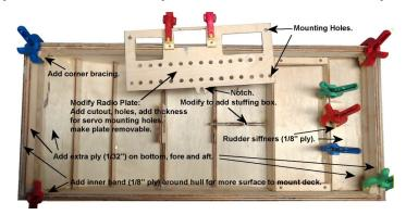
Once everything was installed in the hull (motor, battery, radio, speed controller, rudder servo, rudder post and drive shaft it was time to install the deck. I did not use the supplied deck or pilot house as it would not work with the design I opted for.
