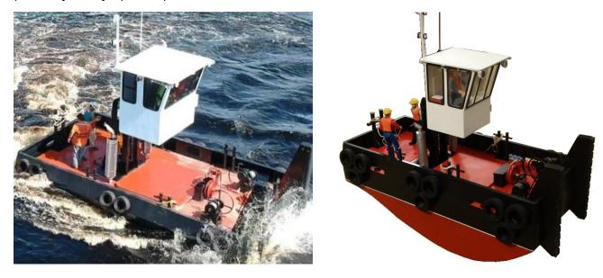
Above you can see the real versus the model of the pushboat. The pilot house raises and lowers using a belt and cogs from the disposed ink jet printer. The drive is that
