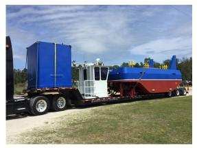
The pushboat here is in three pieces, the hull on the back of the trailer, the mid section house (blue box) on the front, and the pilot house in the middle.
