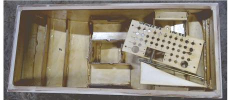
the receiver and speed control in place by using plastic ties.
